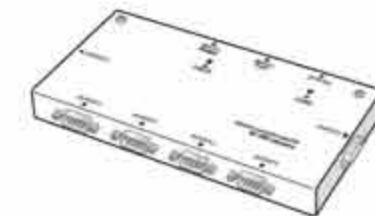
RS-232C Distributor (1-in 6-out, essential for config. over 3x3)
